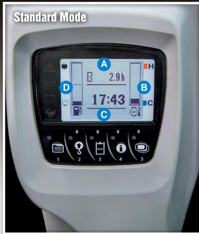
With easy access, simple settings, and easy-to-read indicators and alerts, you'll always be aware of the status of your excavator's critical functions. The wider, more visible display screen with easy push button operation puts convenience at the operator's fingertips. Part of Kubota's Intelligent Control System, the digital panel provides a wealth of user-friendly information to help keep the KX033-4 working safely and efficiently.
