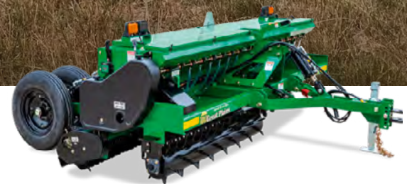
BROADCAST SEEDER 2.2m to 3.3m working width
