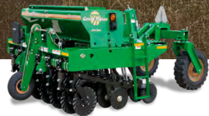
MOUNTED NO-TILL DRILL 1.7m to 2.9m working width
